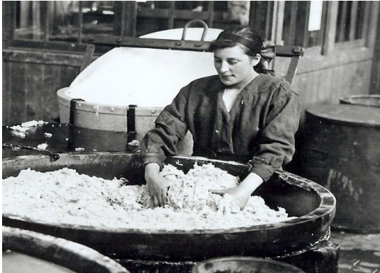
A munitions worker unloading the nitrating pans at HM Factory Gretna. This mixture of 'Devil's Porridge' was highly explosive and very dangerous.
