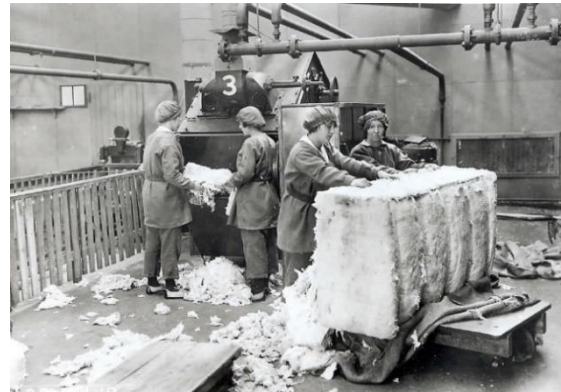
Munitions workers turned raw cotton into Cordite needed for bullets and shells. Munitions workers broke up bales of cotton, a key ingredient for making explosive cordite.
